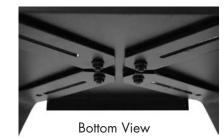
3. Align remaining holes on Grill Support Base with Cart Legs. Insert 4 Carriage Bolts into **outer holes** on Top Base connecting it to Cart Legs with Nuts. **WRENCH TIGHTEN** <u>ALL</u> **CONNECTIONS.**
